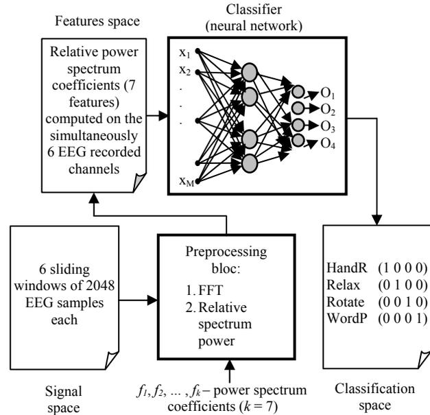
Fig. 1. System data flow schematic
